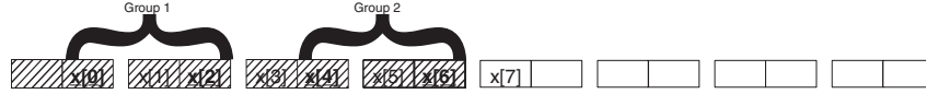
Fig. 5. Irregular access to 2 groups of 3 elements separated by a distance 4 with a probability 0.57 of array x .
